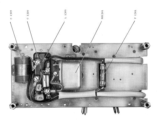
Figure 9 24VDC Power supply
