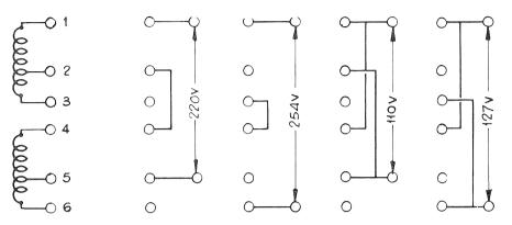
The transformer TR1402 supplies all voltages to the transmitter except filament voltage, and this transformer is connected, when either the button SIMPLEX or the button DUPLEX is pressed.
