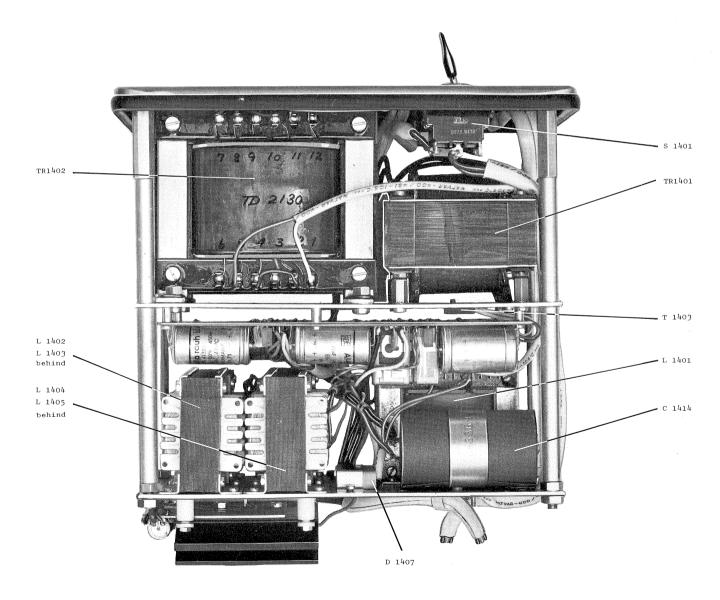
Figure 7 220/110 VAC Power supply
